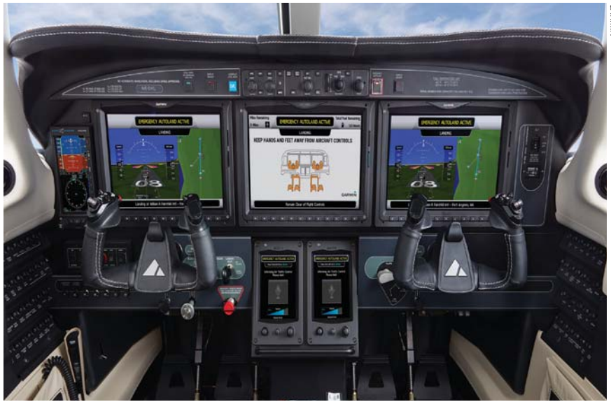
Pressing the red "No Panic" button activates a simple audio-visual passenger briefing system, instructing them what to do, how to communicate with ATC, if needed, and where they are being flown.
