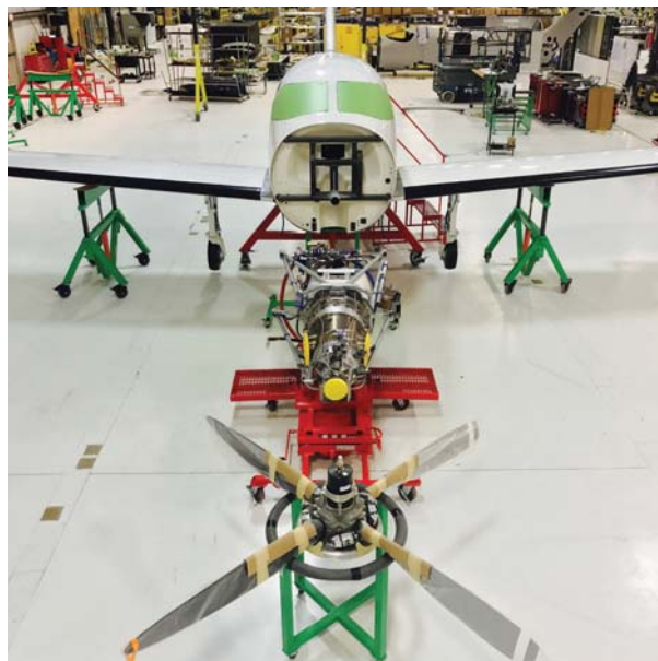
The E1000’s PT6A-67A engine is rated at 1,200 hp for 5-min. takeoff limit. Having the highest power-to-weight ratio of any single-engine turboprop in BCA’s June 2019 Purchase Planning Handbook enables the aircraft to take off over a 50-ft. obstacle in 2,252 ft.
